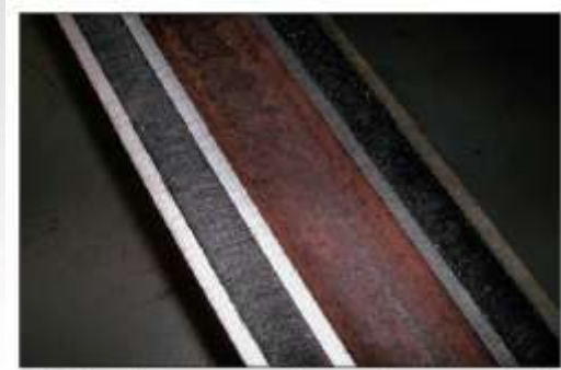
4.2-in.-OD pre-expansion packer expanded in 4.9-in.-ID test fixture
